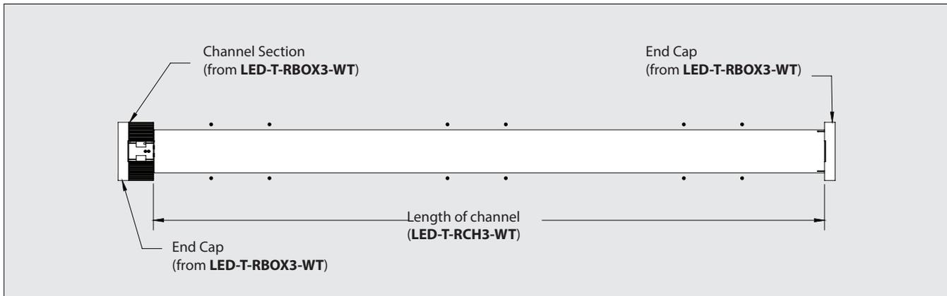
8. If required for installation, cut down **LED-T-RCH3-WT** to measured/desired length with hacksaw or miter saw that has an appropriate blade for cutting aluminum. Always wear safety goggles when cutting. (Note: Channel should be cut together with the diffuser to ensure proper fitting.)
